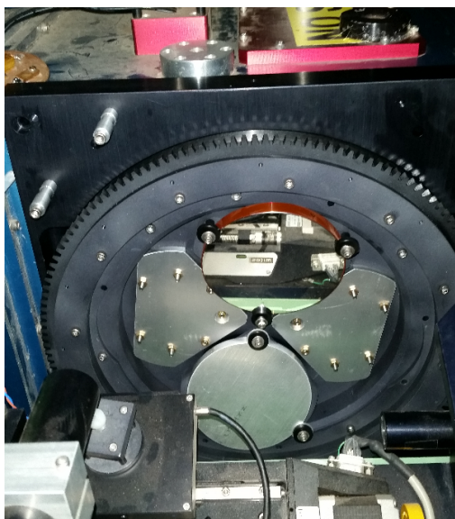
Figure 3.4: UBC entrance window rotator with only the LBTI window (top) installed. See description in Sect. 3.2.2.
