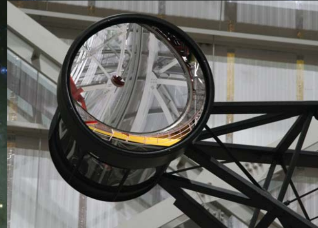
An adaptive secondary mirror (ASM) reflecting its primary mirror. On the picture opposite, each ASM can be seen hanging from the highest arm on each side of the telescope.
