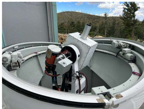
A view inside the SDI dome showing the PEPSI SDI (far side) with the new RINGSS telescope (near side, left) and iLocator solar feed (near side, right) sharing a common robotic mount. Photo credit: I. Ilyin
